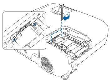
Replace the lamp cover and tighten the screw to secure it.
