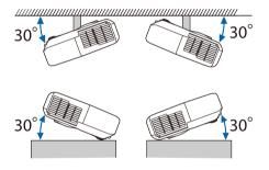
If you use the projector tilted at an angle of more than  $30^{\circ}$  it could be damaged and cause an accident.
