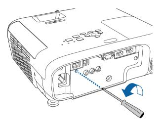
**2** Connect the wireless LAN module to the USB-A port.
